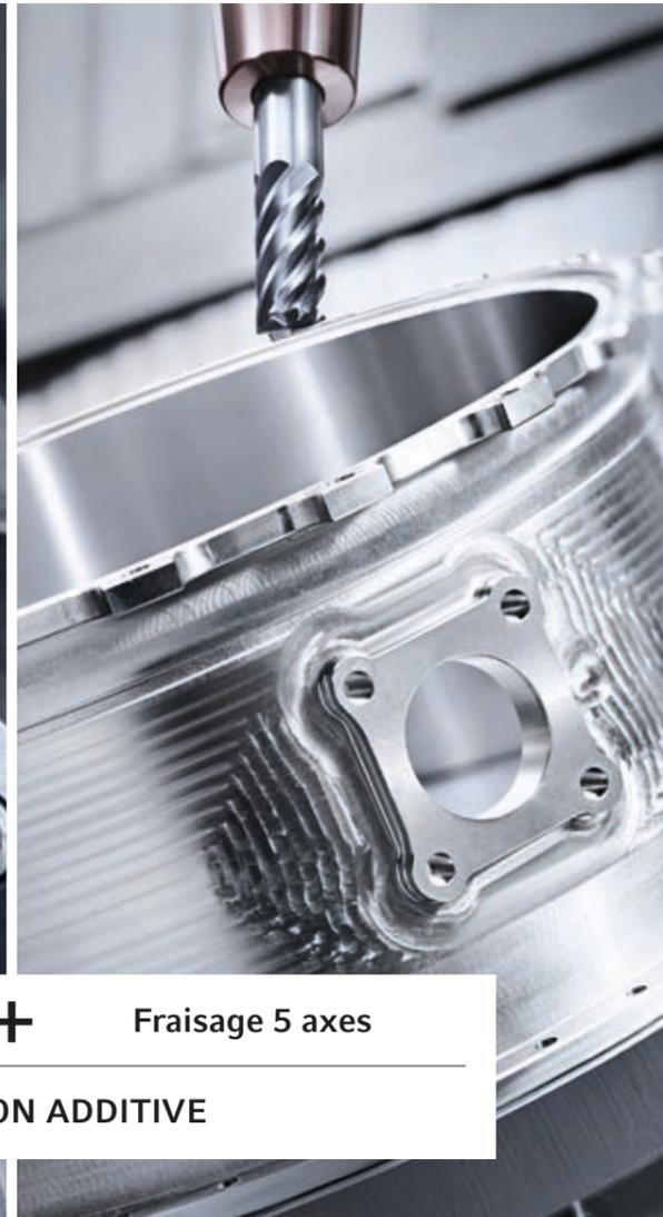
Rechargement laser + Fraisage 5 axes
